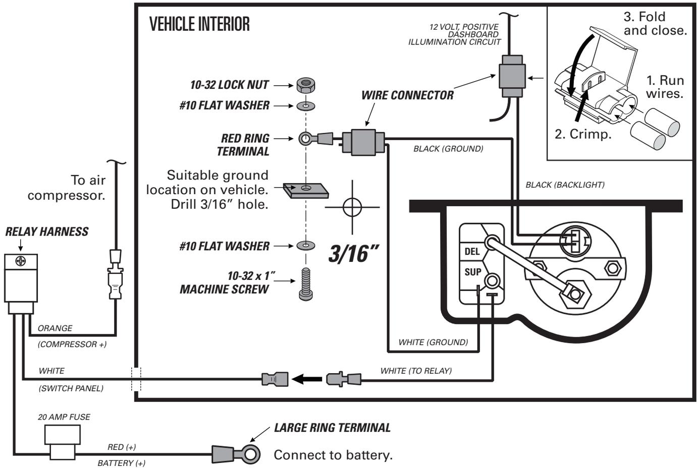
**3** Install the control panel using the supplied fasteners.
