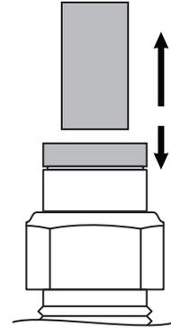
**Removal Tip:** Use a 1/4", 5/16", or 6mm open-ended wrench to push the collar down.
