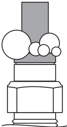
Release air line tube (see page 4). Review proper cuts and procedures in step 5. Repeat installation steps.
