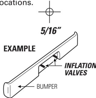
**3** Install Inflation Valve assembly as shown.
