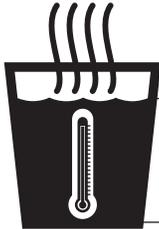
FOR PROPER INSTALLATION, SOAK AIR LINE TUBE ENDS IN HOT WATER BEFORE INSTALLING ONTO BARBED FITTINGS.
