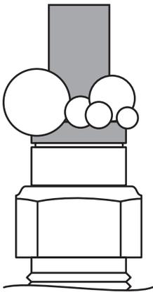
Release Air Line Tube (see page 11). Review proper cuts and procedures in Step 9. Repeat Steps 10 and 12.
