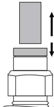
**Removal Tip:** Use a 1/4", 5/16", or 6mm open-ended wrench to push the collar down.
