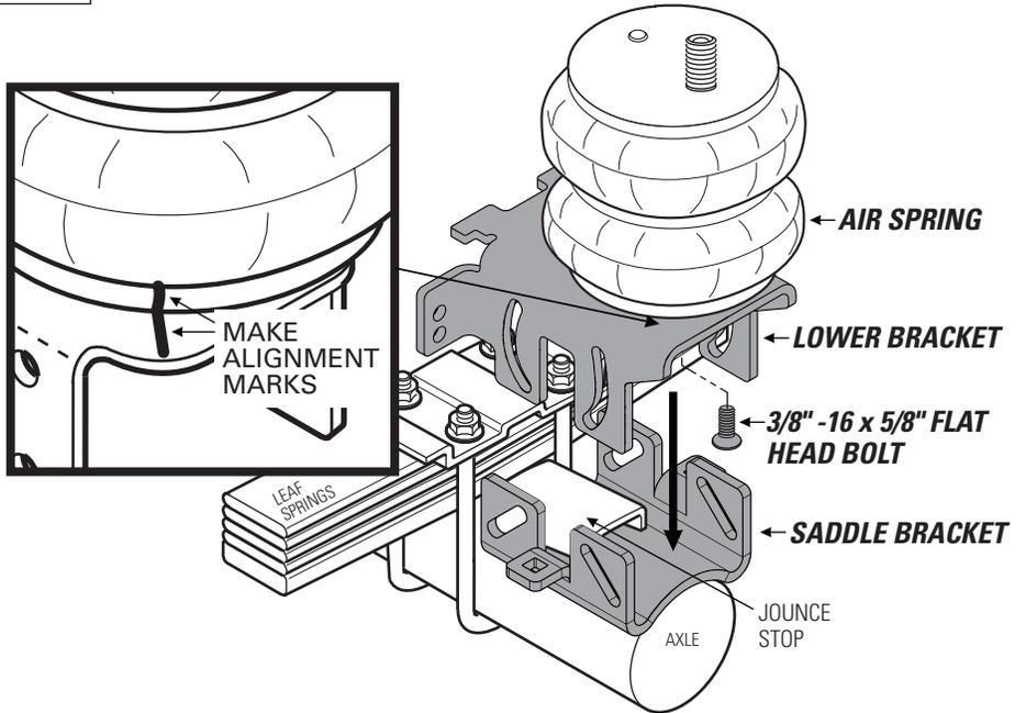
**5** Position the Lower Bracket as low as possible, while still clearing the jounce stop on the vehicle.
